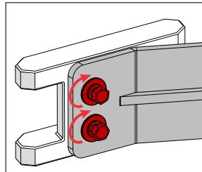
Align the ladder and tighten the bolts.
