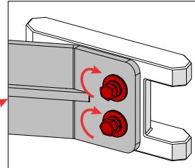
Align the ladder and tighten the bolts.
